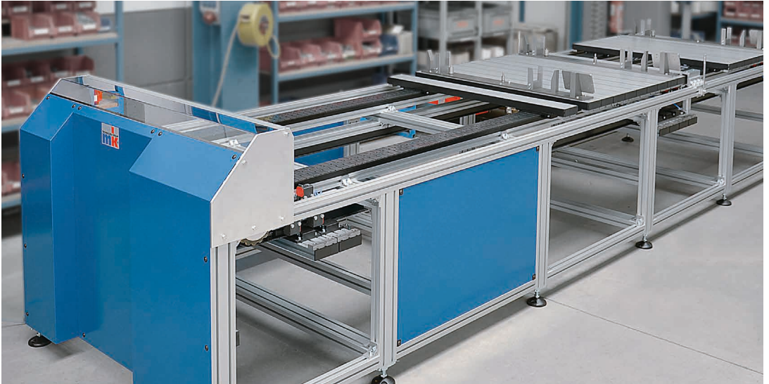
SPU 2040, double-line with separating function for supplying parts in an assembly and welding facility
