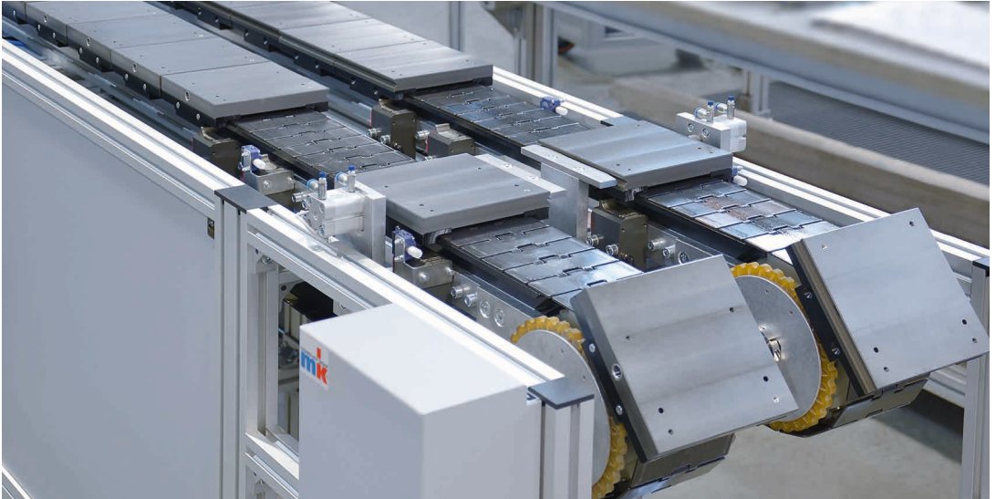
SPU 2040, dual-line, 114 chain width with positioning unit
