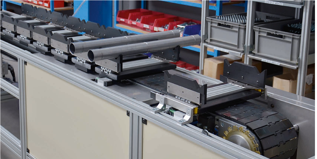
SPU 2040, single line with pallet separating function for supplying parts in a production facility
